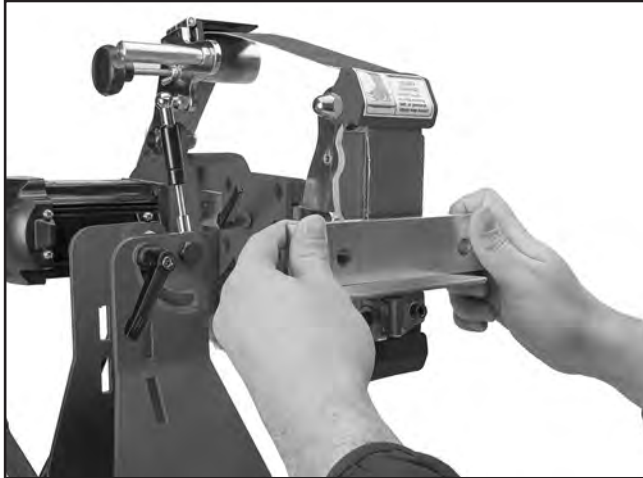
Figure 40. Properly grinding workpiece face.
