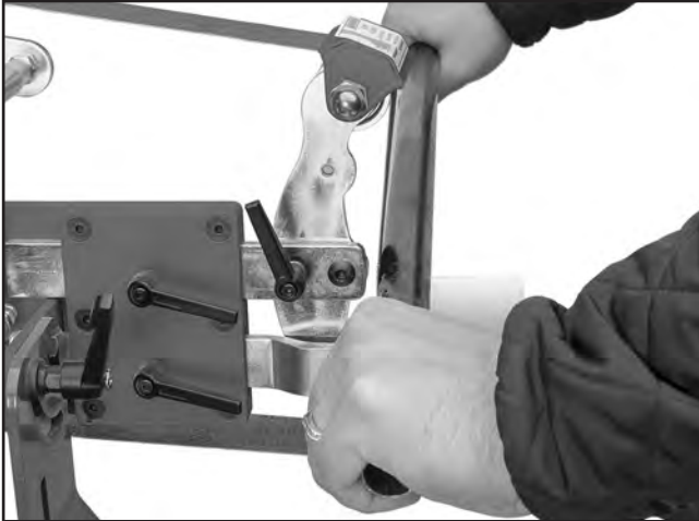
Figure 41. Example of slack belt grinding.
